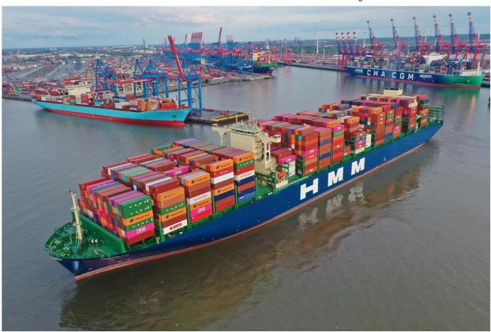
All eight ships in the series are of the largest possible neo-Panamax design capable of transiting the expanded Panama Canal and are fitted with scrubbers to allow the use of high sulphur fuel oil.
