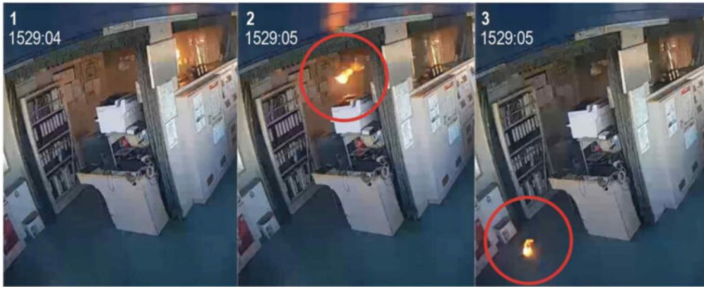
Photos from the bridge closed-circuit camera showing (1) a second explosion, (2) an object on fire propelled into the air (circled in red), and (3) the object, still on fire, landing on the floor (circled in red). (Background source: Stalwart Management Ltd)
