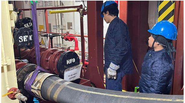
A Maersk vessel is bunkering bio-diesel in the port of Rotterdam. This green fuel comes solely from waste streams and reduces the Greenhouse Gas (GHG) emissions by more than 80% compared to conventional fossil fuels.
